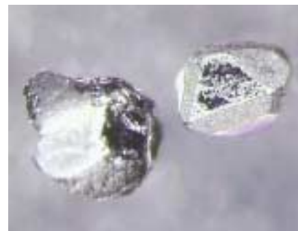
Chromite grains from sample FX-241. Grains are 0.3 mm across. (Photo 48401)
