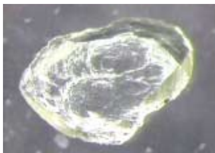
Olivine grain (0.3 mm across) from sample FX-210. Note the well preserved crystal edges. (Photo 48403)
